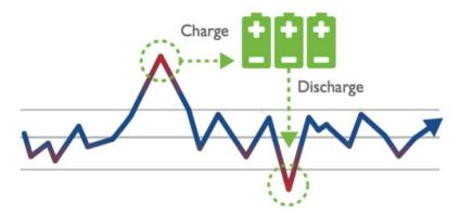
The UK electricity grid is maintained close to a frequency of 50Hz.
